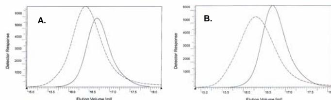
SEC of A. PDLA-*b*-PDMAEMA (dashed line) and PDLA-Br macroinitiator (solid line) and B. PLLA-*b*-PDMAEMA (dashed line) and PLLA-Br macroinitiator (solid line).
