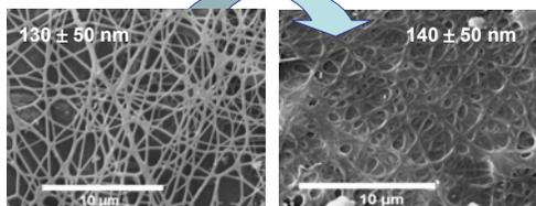
Yarns formation from self-assembled fibers during the electrospinning process from chitosan/PAMPS/HCOOH/CaCl<sub>2</sub> system using a static collector [3]
