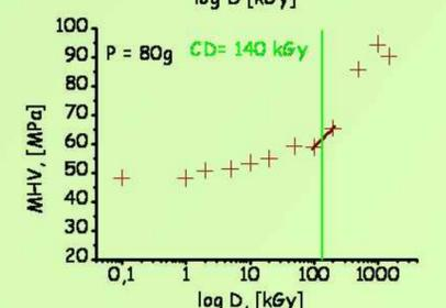
Fig. 4. Effect of the irradiation dose on the Vickers microhardness (MHV).
