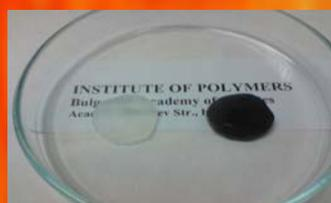
Macroporous nanocomposites are obtained by mixing high molecular weight PEO with PAAm-grafted MWNTs in aqueous media, freezing at minus 20 °C and subsequent freeze drying.
