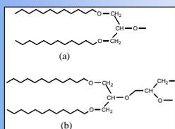
Fig. 1. Chemical structures of the lipid-mimetic anchors: 1,3-didodecyloxypropane-2-ol (DDP), (a); 1,3-didodecyloxy-2-glycidyl-glycerol (DDGG) (b).
