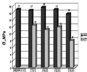
Fig. 1. Tensile strength of NBR- (black bars) and EPR-containing (grey bars) blends
