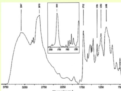
**Fig. 4.** IR spectrum of 4. The IR spectrum of 4-ethenyl-1,3-dioxolan-2-one in the region 2000–1200 cm<sup>-1</sup> is presented
