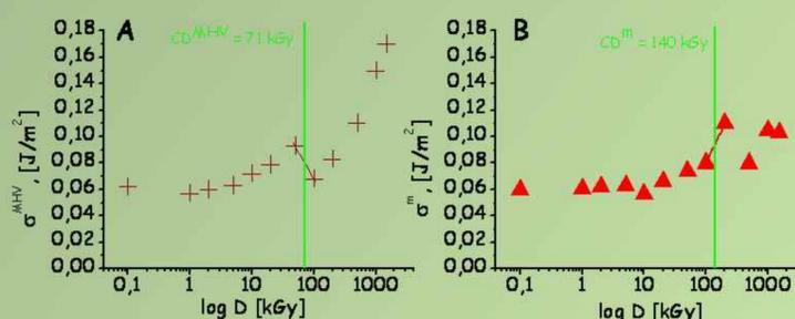
Fig. 2. Effect of the irradiation dose on surface free energy, estimated by MHV (A) and kinetics of non-isothermal melting (B)
