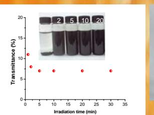
Influence of the irradiation time on the grafting efficiency at NIPAAm:MWNTs mass ratio 400:1
