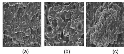
Fig. 5. SEM morphology (x1000) of (a) cryogenic fractured surface of LDPE/PP blend (1:1); (b) triple LDPE/PP (1:1) blend containing 12.5% NBR and (c) triple LDPE/PP (1:1) blend containing 12.5% EPR
