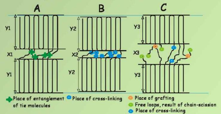
Fig. 1. Changes in polymer structure caused by  $\gamma$ -irradiation: A - lamellar structure of unirradiated sample; B - lamellar structure of irradiated sample during radiation annealing; C - lamellar structure of irradiated sample during radiation melting.  $Y_1, Y_2, Y_3$  - thickness of lamellae:  $Y_1 = Y_2 = Y_3$ ;  $X_1, X_2, X_3$  - thickness of amorphous region:  $X_1 > X_2 < X_3$
