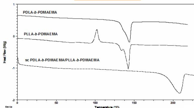
DSC curves of PDLA-*b*-PDMAEMA, PLLA-*b*-PDMAEMA and stereocomplexed "sc" PDLA-*b*-PDMAEMA/PLLA-*b*-PDMAEMA [PDLA-block/PLLA-block = 1/1 (mol/mol)] films cast from  $CH_2Cl_2$ . Heating rate  $-10^\circ C/min$  under  $N_2$  flow. First heating run.
