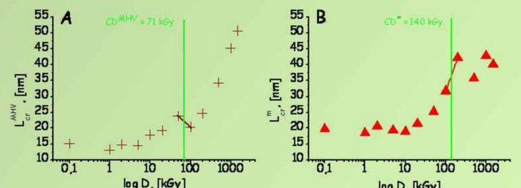
Fig. 3. Effect of the irradiation dose on thickness of lamellae, estimated by MHV (A) and kinetics of non-isothermal melting (B)
