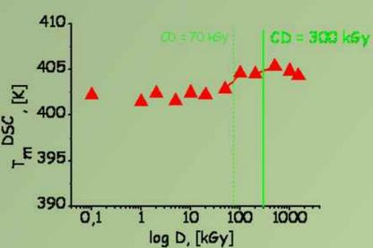
Fig. 6. Effect of the irradiation dose on melting temperature, estimated by DSC
