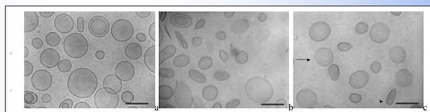
Fig. 4. Cryo-TEM images of samples based on DPPC:Chol at molar ratio 2:1 stabilized by (DDGG)<sub>2</sub>(EO)<sub>112</sub> and (DDGG)<sub>4</sub>(EO)<sub>114</sub>: a) 2.5 mol % (DDGG)<sub>2</sub>(EO)<sub>112</sub>; b) 7.5 mol % (DDGG)<sub>2</sub>(EO)<sub>112</sub> and c) 7.5 mol % (DDGG)<sub>4</sub>(EO)<sub>114</sub>. Arrow shows "flat liposome" in face-on position and arrow head shows "flat liposome in edge-on position. Bars = 200nm
