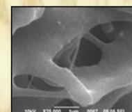
Scanning electron microscopy images of PAAm/MWNTs macroporous nanocomposites at different magnifications
