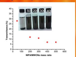
Influence of the NIPAAm:MWNTs ratio on the grafting efficiency at 10 min irradiation with UV light
