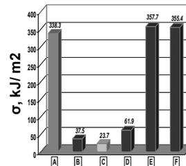
Fig. 6. Charpy impact strength of blended recyclates: [A] -LDPE-recyclate; [B] -PP-recyclate; [C] -LDPE/PP(1:1) -recyclates; [D] -LDPE/PP(1:1) -virgin polymers; [E] -LDPE/PP(1:1)-EPR(15%) -recyclates; [F] -LDPE/PP(1:1)-EPR(20%) -recyclates
