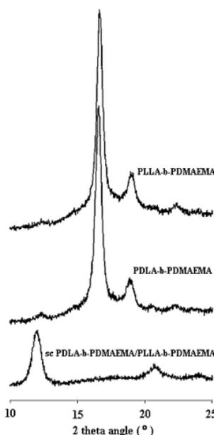
XRD traces of PLLA-*b*-PDMAEMA, PDLA-*b*-PDMAEMA and "sc" PDLA-*b*-PDMAEMA/PLLA-*b*-PDMAEMA films.
