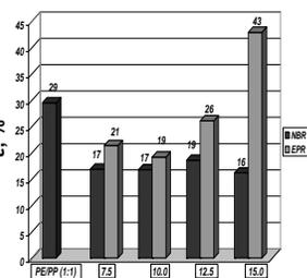
Fig. 2. Elongation of NBR- (black bars) and EPR-containing (grey bars) blends
