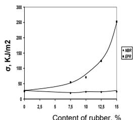
Fig. 3. Charpy impact strength (σ<sub>i</sub>) of PE/PP blends (1:1) with different content of rubber
