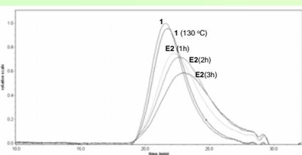
**Fig. 3.** GPC traces of: 1 – starting poly(oxyethylene H-phosphonate); 1(130 °C) – poly(oxyethylene H-phosphonate) after melting at 130 °C, and of the reaction mixture of 4-ethenyl-1,3-dioxolan-2-one and 1 under the conditions of Experiment 2: E2(1h) – after 1 h reaction time; E2(2h) – after 2 h reaction time; E2(3h) – after 3 h reaction time
