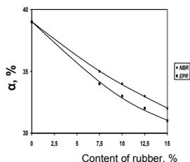
Fig. 4. Influence of the content of rubber on the degree of crystallinity (δ) of the blends
