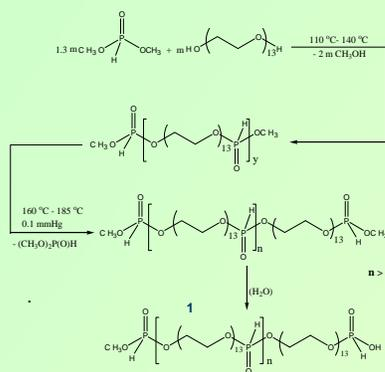
**Scheme 1.** Reaction pathway used for preparing the poly(oxyethylene H-phosphonate)
