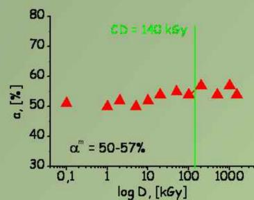
Fig. 5. Effect of the irradiation dose on degree of crystallinity, estimated by DSC
