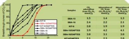
Figure 5. CO 2 breakthrough curves of the modified and parent materials under dynamic conditions.
