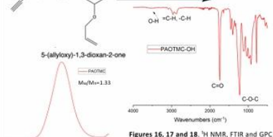
Figures 16, 17 and 18. 1 H NMR, FTIR and GPC spectra of the obtained polymer. 1 H NMR is done in CDCl 3 at 600 MHz.
